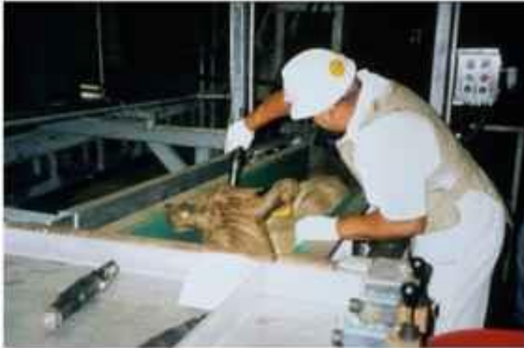
Captive bolt stunning in center track restrainer
